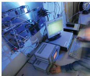
Different catalytic converters can be characterized and compared under repeatable conditions on the IAV synthetic gas test bench
