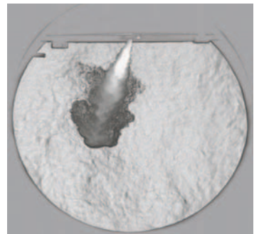
Fig. 4: Spray pattern of a multiple-hole injector, taken in IAV's pressure chamber using the Mie / Schlieren method for the simultaneous visualization of vapour and liquid distribution
