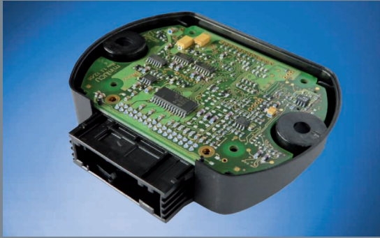
BMS control unit (master)
