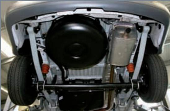
Packaging of underfloor LPG tanks
