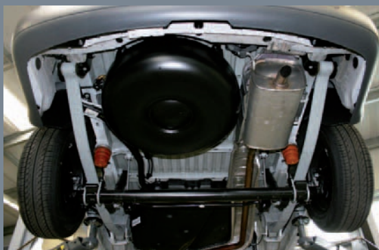
Packaging of underfloor LPG tanks
