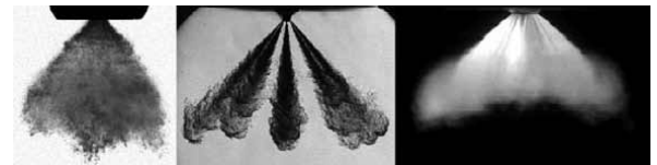
Visualization of injection through a swirl, multi-hole and ring-gap nozzle
