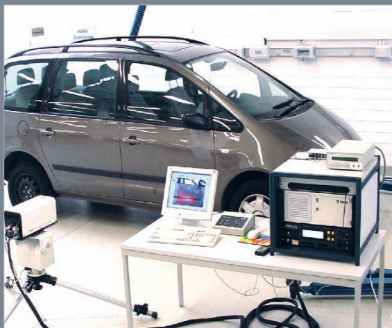
Measurement of the surface velocity by laser vibrometry
