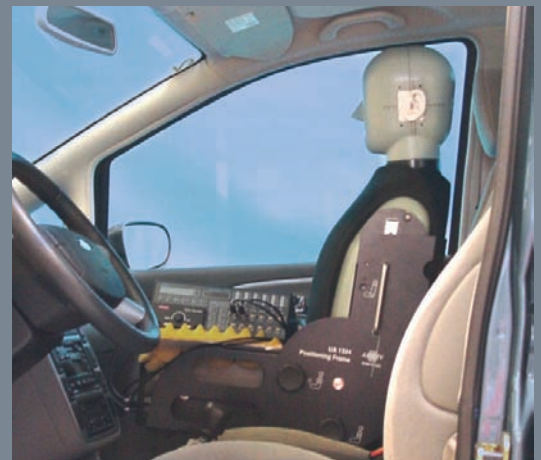
Mobile artificial head measurements for psychoacoustic evaluation
