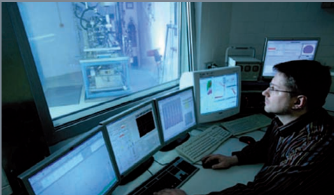
Function testing of injection systems
