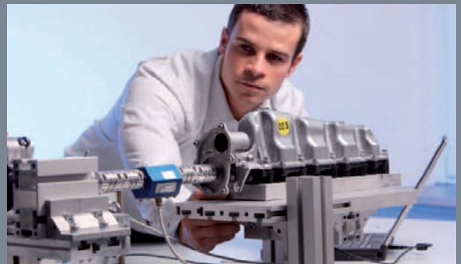
Test bench for flaps and valves
