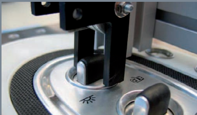
Switch test bench
