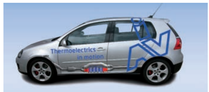
IAV's experimental vehicle for testing TEG systems under real-life conditions in road traffic
