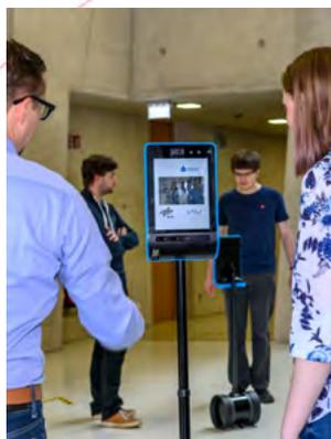
The self-driving robots used in „AI in the loop“ already drive up and down the hallways and can pick up guests from the elevator.
