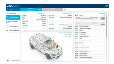
The remote service center makes it easy to ascertain the status or "health" of a vehicle, for example by pulling diagnostic data (DTCs) or measurement data.
