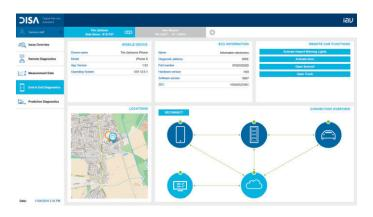
The end-2-end diagnostic function permits online support such as remote lock/unlock, remote heating or A/C analysis to tell the customer exactly what went wrong in the processing chain.
