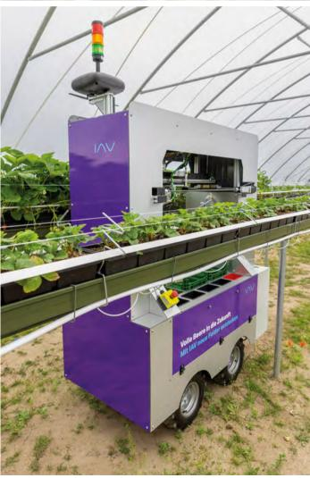
Harvesting robots in action: With the latest sensor technology autonomously on the move in planting aisles. The gripper arm locates the strawberries, classifies them according to ripeness and carefully separates the fruit.
