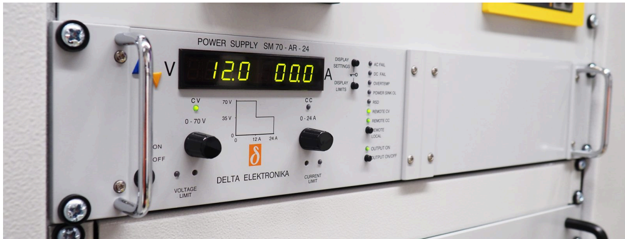
HV power supply inside the IAV Auros Iso. The DC component comes from the power supply, the AC component from the ripple generator.
